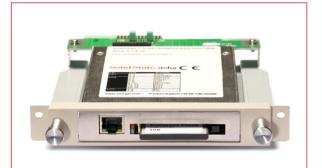
Floppyflash replacing the NEC 3.5in 1.44MB Bezeless Slim Floppy Drive FD1238T
