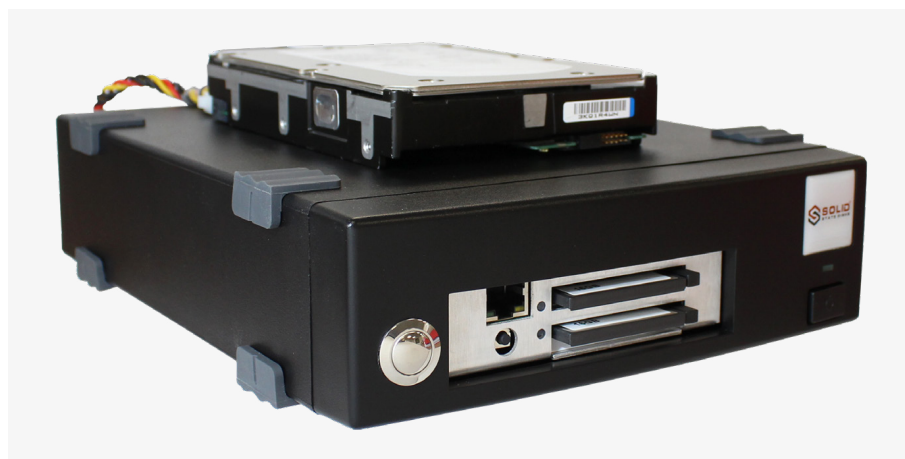
Figure 1: A legacy SCSI HDD (top) being cloned to a CF card using DuplicatorPlus - the card can then be used in a SCSIFlash drive, which presents a form-fit-function replacement of the HDD
