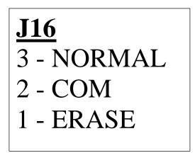
Fit J16 pin 2-3 for normal operation. Fit 1-2 to erase software.
