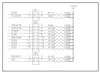
For current operation the following links should be fitted.
