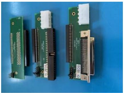
Note SCSI ID on 68 and 50 pin adaptors and not on 80 pin adaptors.
