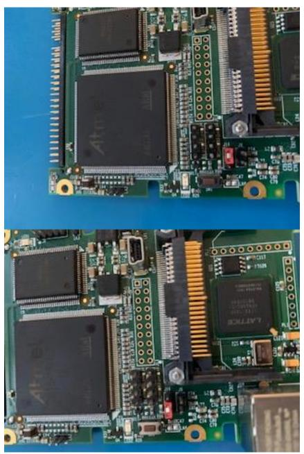
**Note:** if the SF250 is not erased the com port will not show when connected by USB and the Heart Beat LED will still be flashing.
