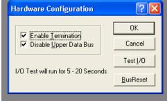
Make sure both boxes are ticked. If the drive that the analyser connects to, real or emulator, has termination fitted then it should be removed if possible because termination moves over to the analyser when the box is ticked.
