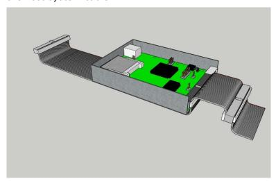
Connect the Analyser pod using the 68 to 50 pin adaptor as follows
