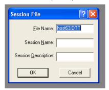
Type in a suitable name for the capture file. Don't worry about adding the .DTT extension SCSIView will add that for you. SCSIView will also add a number each time a capture is run so that you don't have to type in a new name each time, just click OK in that case.
